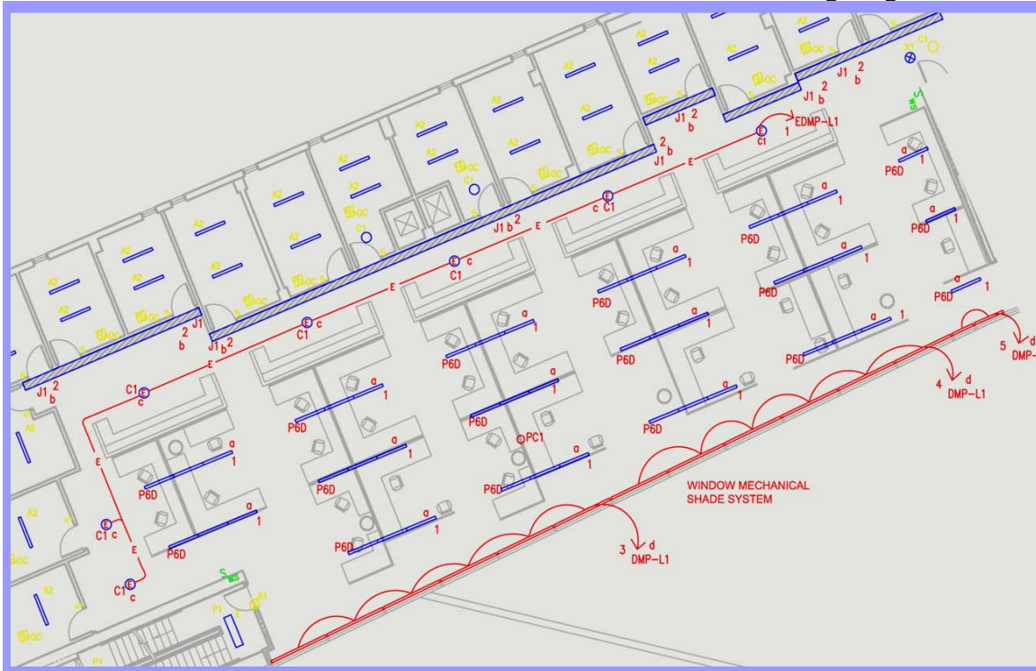
Open Office Lighting Design Circuiting Plan
